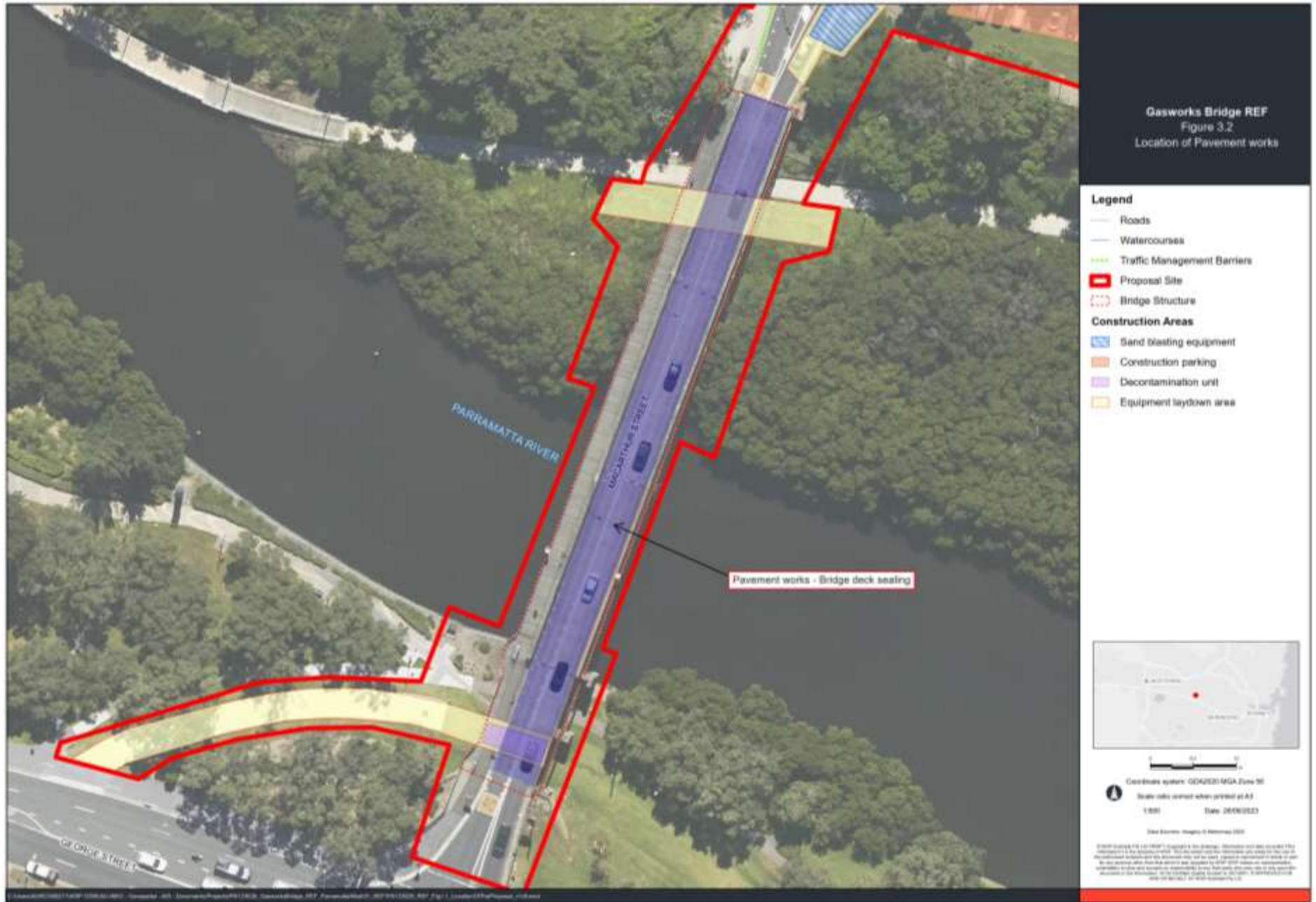
Figure 3.2: Location of the proposed pavement works
