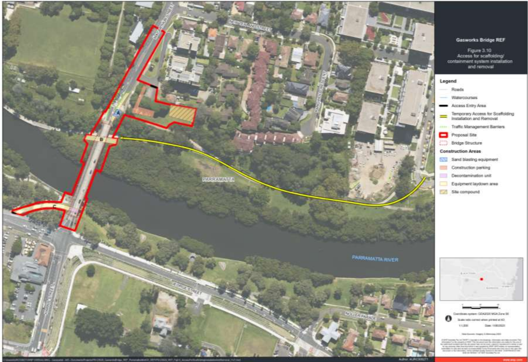
Figure 3.10: Access for scaffolding/containment system installation and removal
