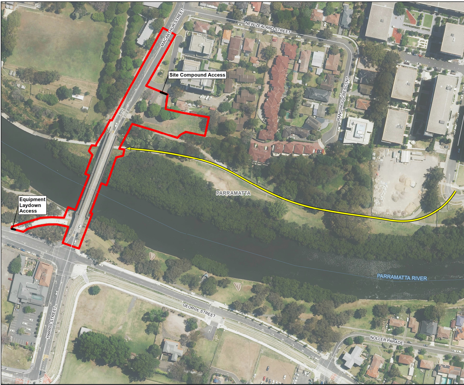
Figure 3.6 Access for scaffolding installation and removal
