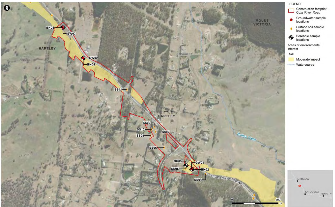
Figure 8.2: Summary of areas with moderate or above contamination risk for CRR study area
