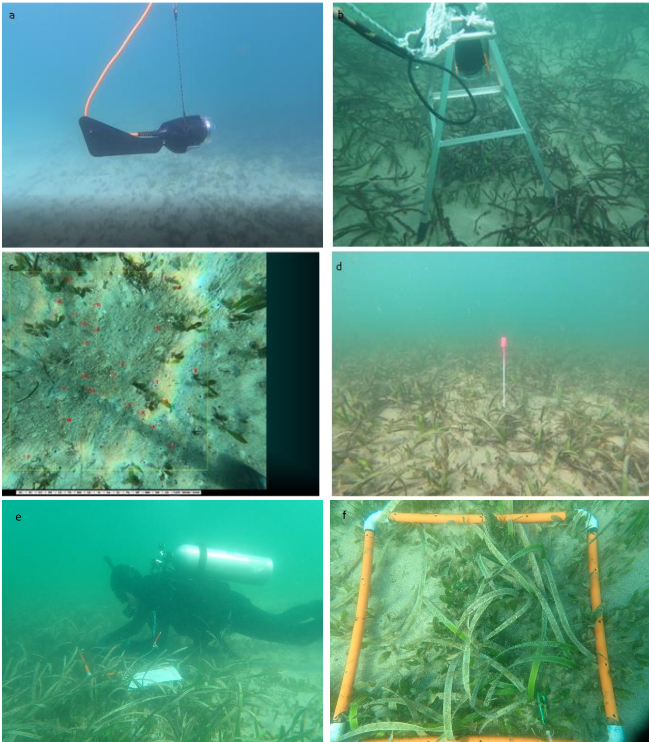
Plate 1: Survey equipment and methodologies a) Towed camera used to map seagrasses, b) Drop camera used to collect photoquadrats, c) CPCe digital photoquadrat analysis screen, d) DoD rod installed within the main P. australis seagrass bed at Kurnell, e) dive survey, f) 0.25 m 2 quadrat.
