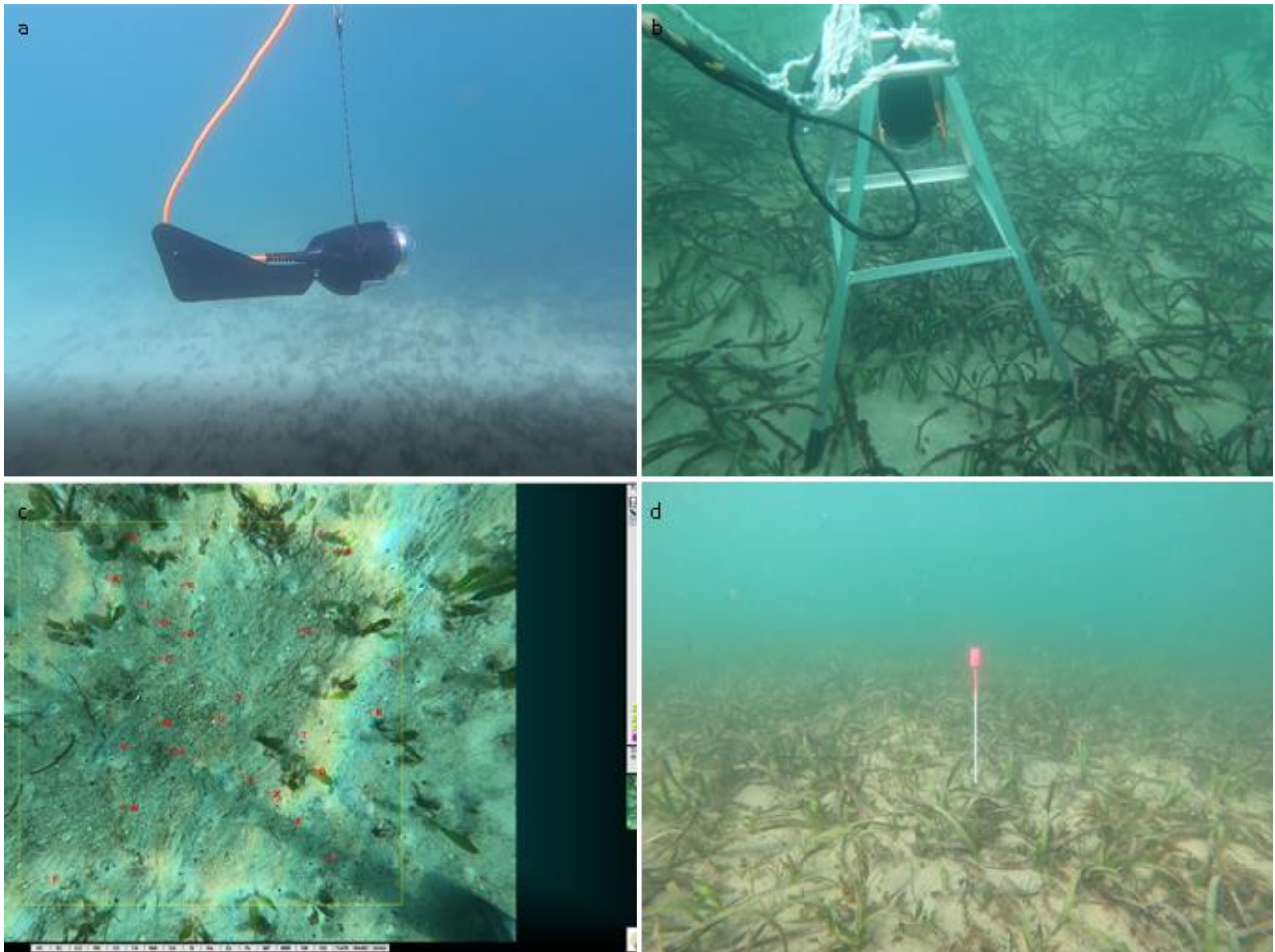
Plate 1: Survey equipment and methodologies a) Towed camera used to map seagrasses, b) Drop camera used to collect photoquadrats, c) CPCe digital photoquadrat analysis screen, and d) DoD rod installed within the main I P. australis seagrass bed at Kurnell.
