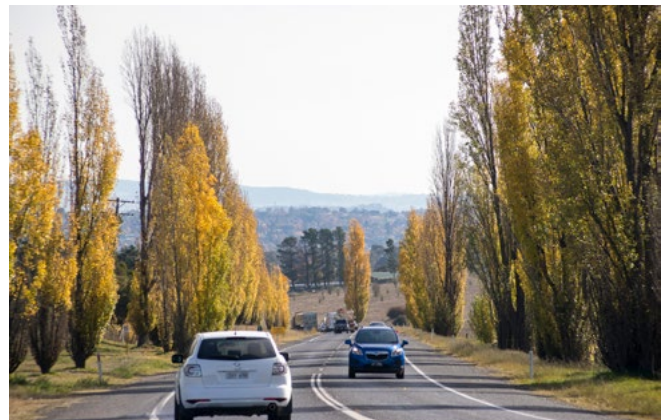
The use of distinctive trees can provide subtle warnings of urban areas ahead as well as differentiate between settlement and rural areas. They help warn motorists of a change in character to an urban area and that slower speeds may be appropriate and required.
