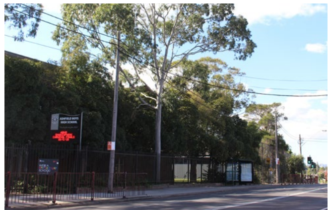
The Eucalypt has been retained by bundling the overhead services so that the clearance envelope is reduced. Note that the side of the trunk which faces the service has been trimmed of branches which may otherwise cause conflict.
