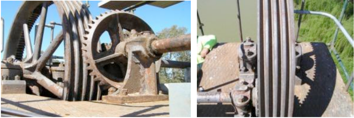
Figure 5.26 2nd motion shaft and sheaves on VIC side down stream (Source: RMS)
