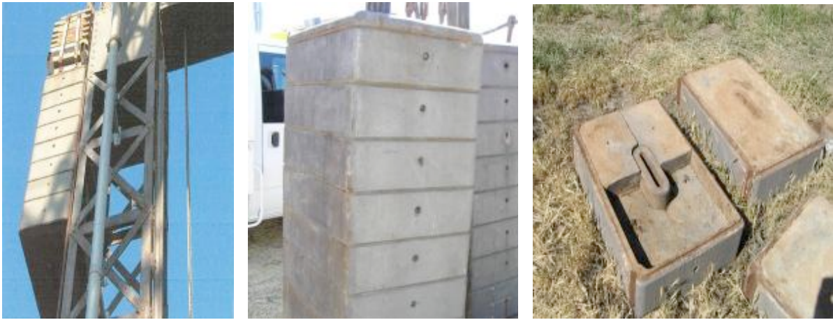
Figure 5.25 Counterweights under evaluation, removed from bridge (Source: RMS)
