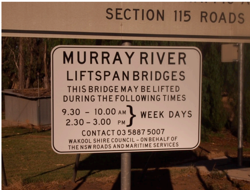
Figure 5.17 Signboard detailing the off-peak traffic times when the lift span can be raised
