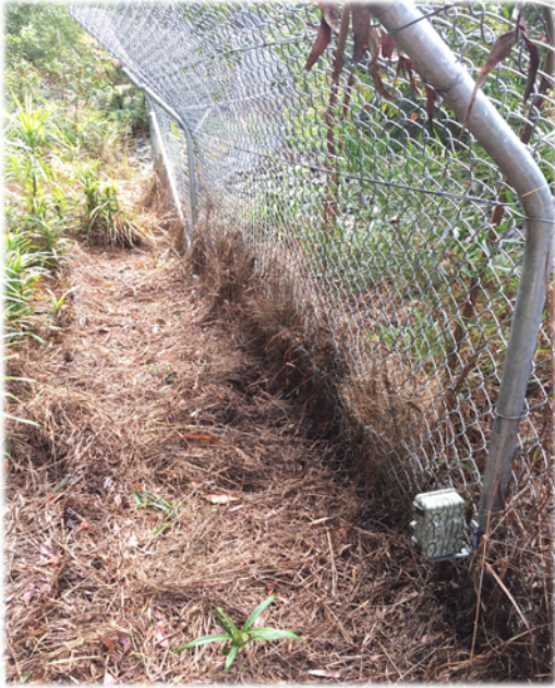
Plate 3: Typical exclusion fence camera set up. It shows a Scoutguard KG680V camera attached to a steel bracket which is fixed to a fence post.
