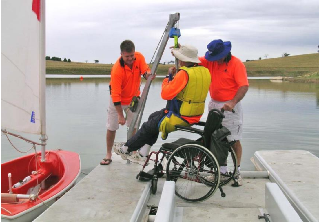
Figure 27: Example of a davit used to achieve all-ability access from a pontoon
