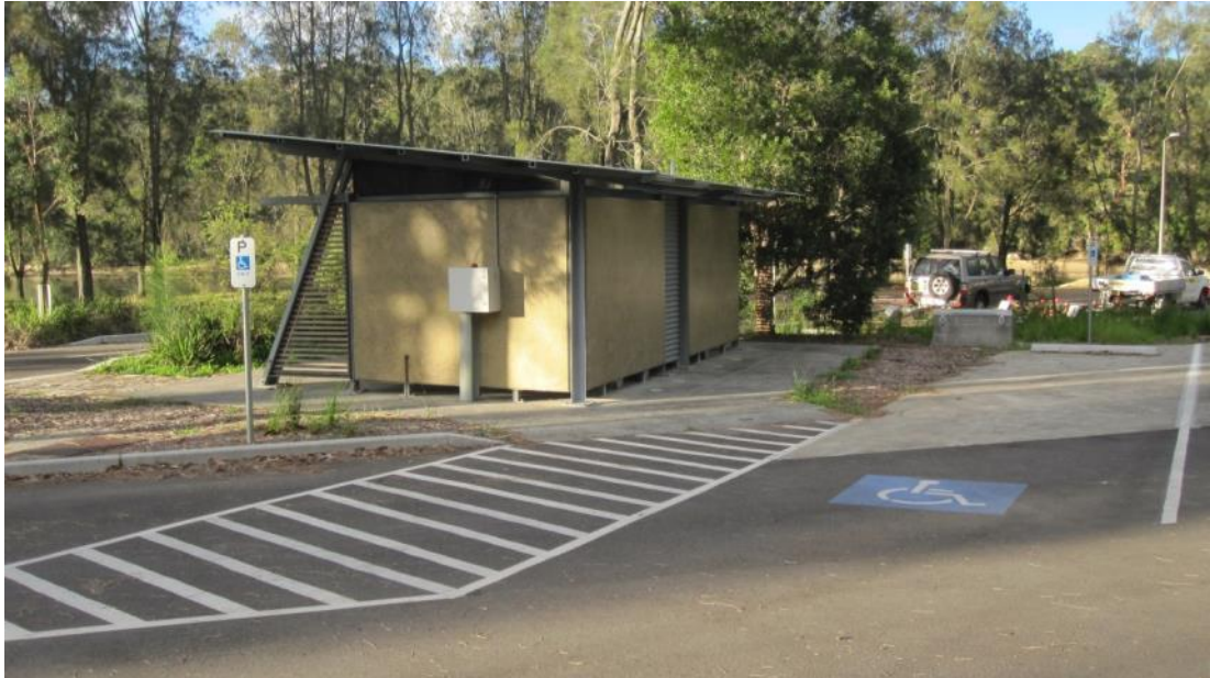
Figure 23: Disabled access car space and shared area in close proximity to amenities block
