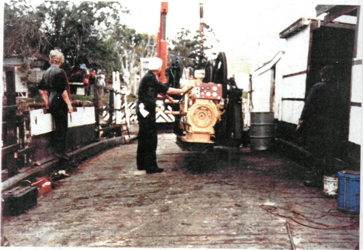
Fitting the old Hibbard ferry with a hydrostatic drive, pre-1984
