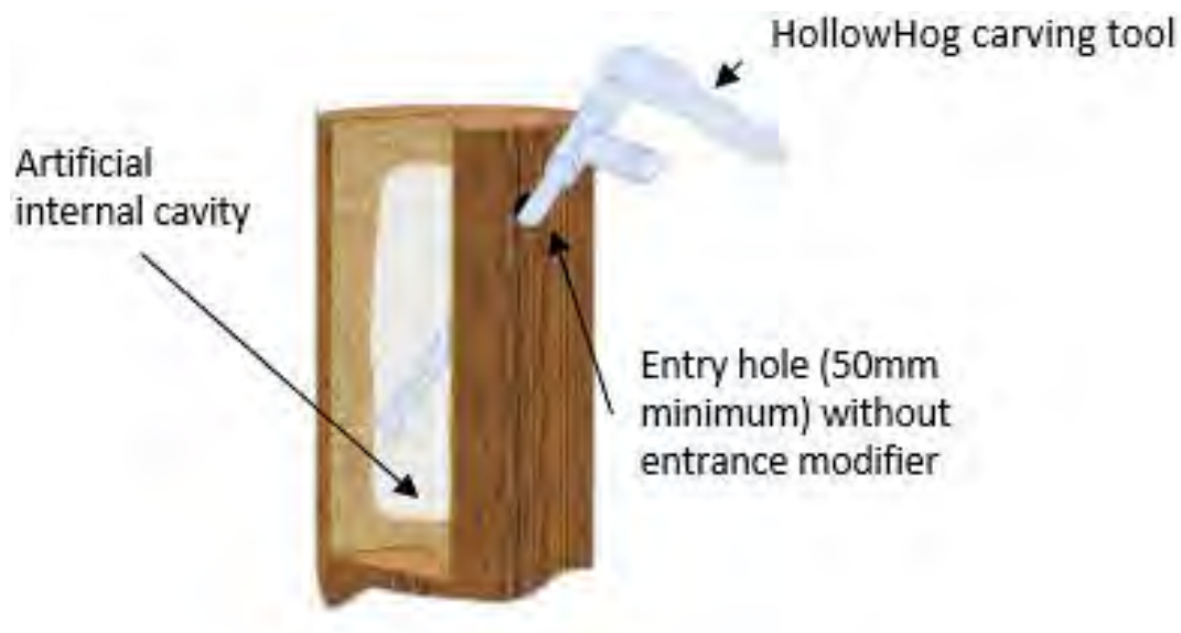
Photo 4.1 Informative diagram of the Hollowhog installation method (HollowHog, 2021)
