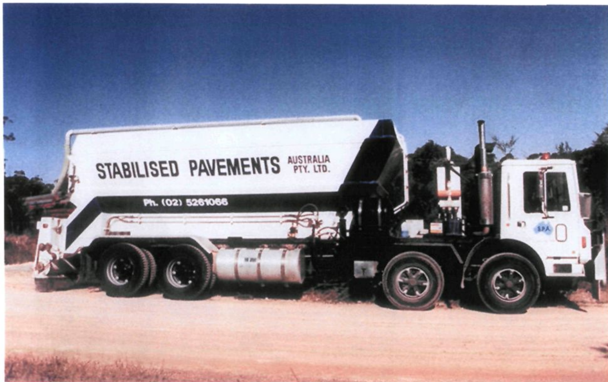
Modern spreaders delivered better uniform spreading than traditional tipper trucks and bags of cement. These units were designed in Australia
