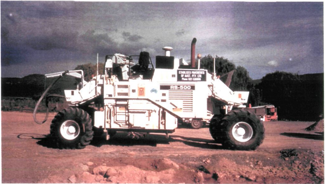
CMI RS-500 was the first of the 'work horses' used in deep-lift insitu stabilisation
