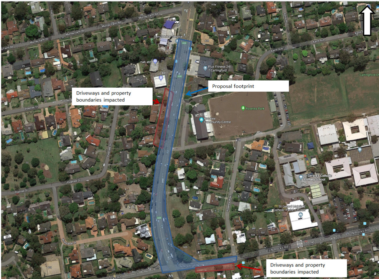
Figure 6-17 Property driveways and fences to be impacted by the proposal that are within the Roads and Maritime road reserve
