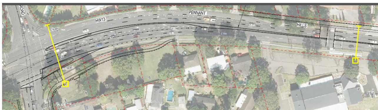
Figure 3-1 Locations of underboring across Pennant Hills Road
