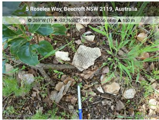
Photo 14. 20.11.2020 Close-up of ACM01.
