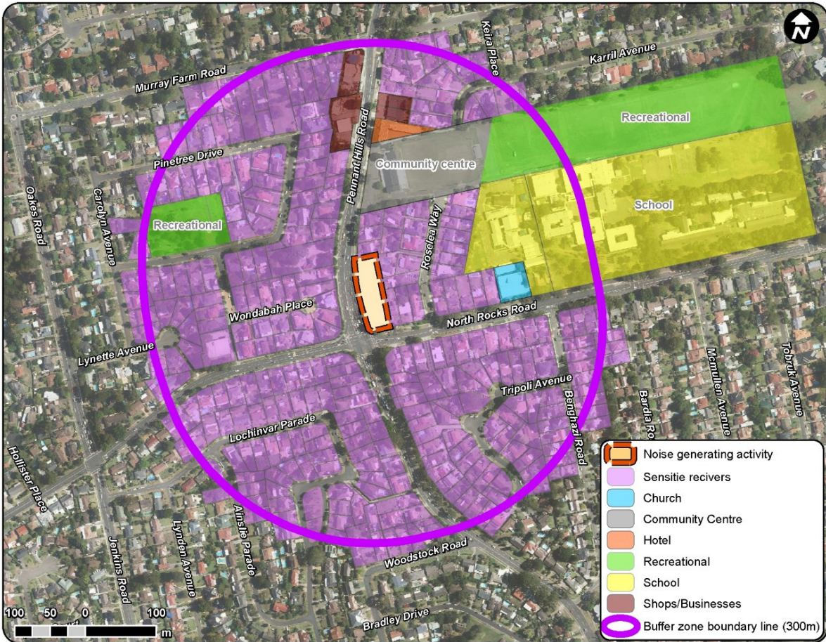
Figure 6-10 sensitive receivers in the vicinity of the compound site
