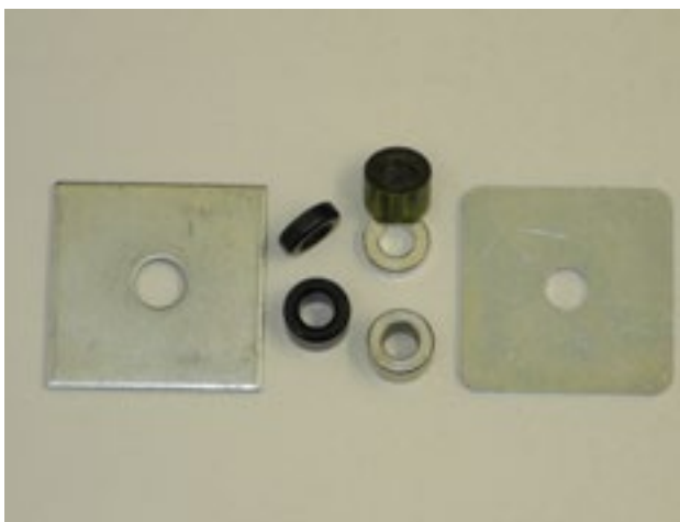
Figure 3-3: Range of parcel shelf spacers (square spacers can be used for Toyota Tarago – between the trim and the body panel – when fitting CRAB).
