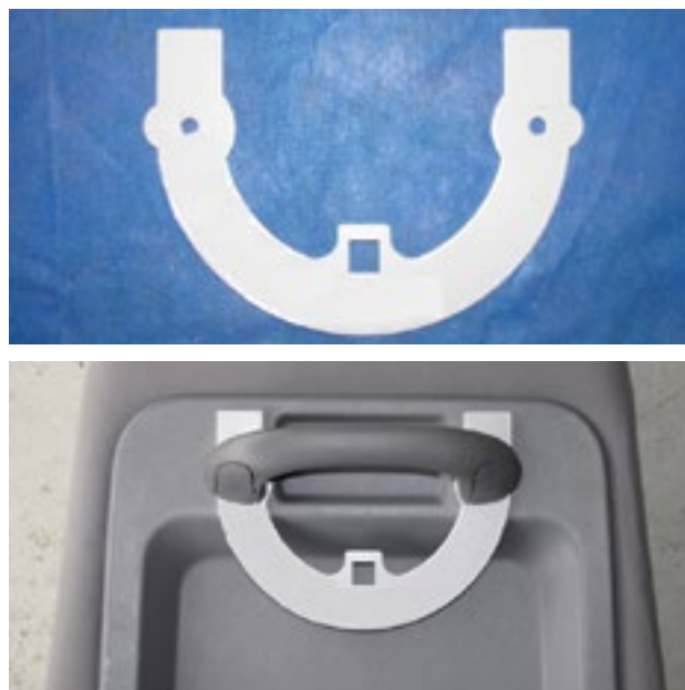
Figure 3-18: Installation bracket for Toyota Commuter (2005 onwards), model A176, and as installed.
