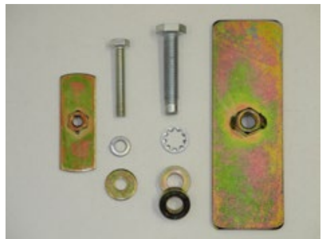
Figure 3-4: Range of spreader plates used for various applications (5/16" UNC thread used for child restraint anchor fittings and 7/16" UNF thread used for seatbelts and CRAB installations).
