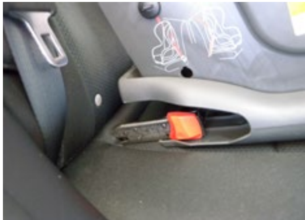
Figure 1-19: Rigid connectors being connected to a vehicle seat
