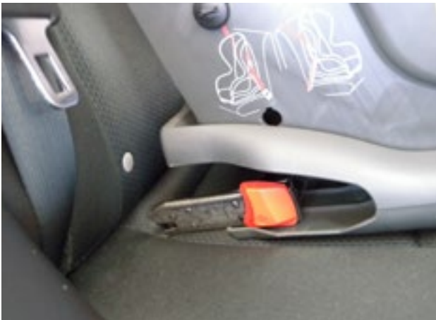
Figure 2-5: Rigid connectors being connected to a vehicle seat.
