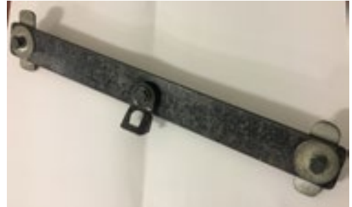
Figure 3-2: Anchor fitting strap to straddle speaker holes (suitable for pre-ADR vehicles).
