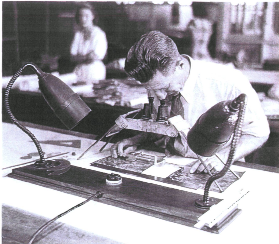
Examining aerial photographs using a stereoscope and stereometer bar, 1949
