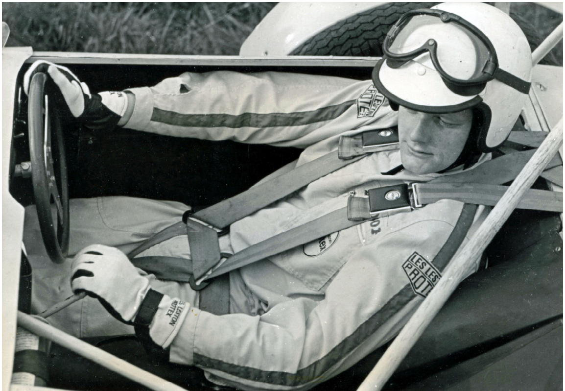
Michael Henderson in his multi-point racing car driver harness (Photo supplied by Michael Henderson)
