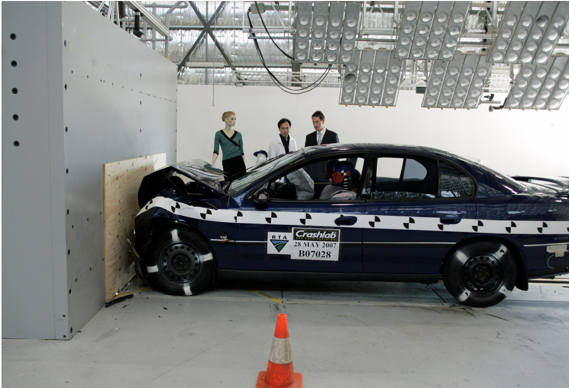
Crash barrier test at Crashlab's Huntingwood facility
