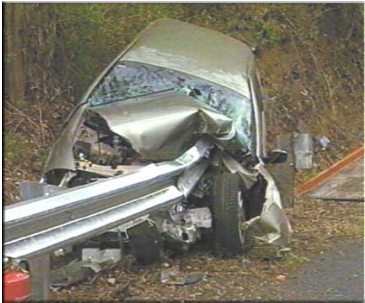
Crash involving steel guard fence (former design)
