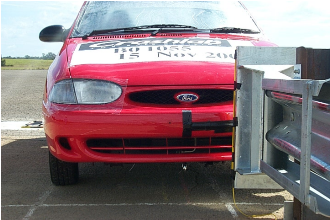
Testing of improved steel barrier terminal
