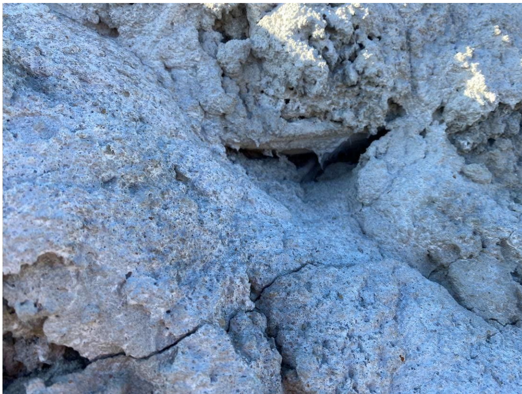
Photo 21. Geofabric marker layer visible in stockpile capping noted in previous inspection 15/05/23 remains. Approximately 5cm x 3cm.
