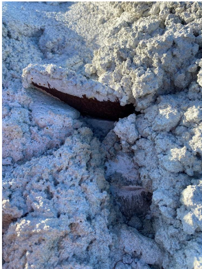
Photo 22. New location of geofabric marker layer visible in stockpile capping. Approximately 2cm x 5cm.
