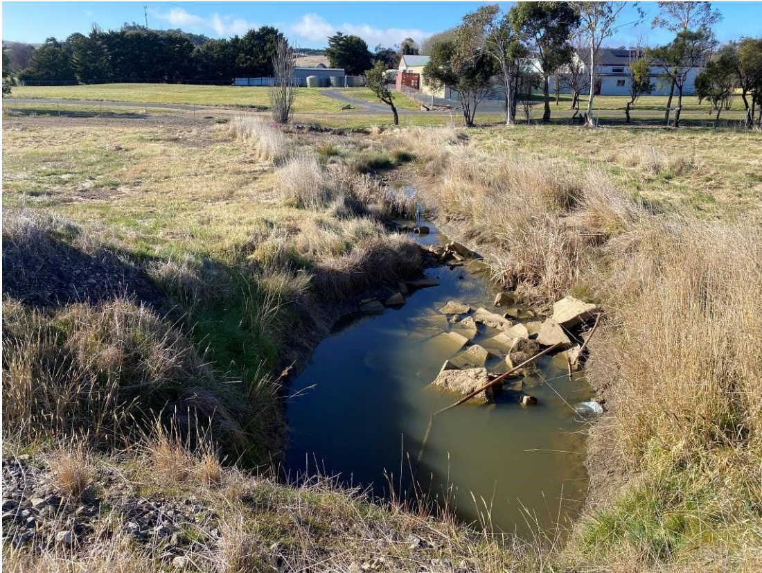
Photo 4: Downgradient of middle culvert showing pooled sediment laden water on site. Sediment has settled more on the bottom of the water body compared to last inspection. Brown, moderate turbidity. No surface water running off site at middle culvert.
