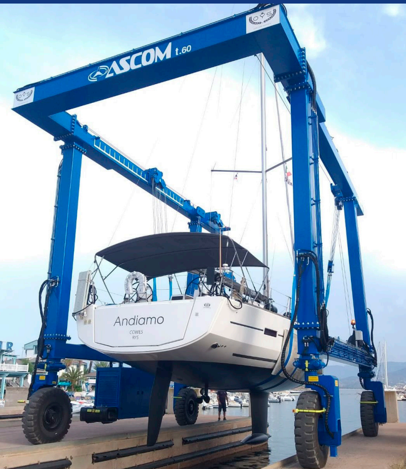
Examples of what the 75-tonne boat travel lift will look like.
