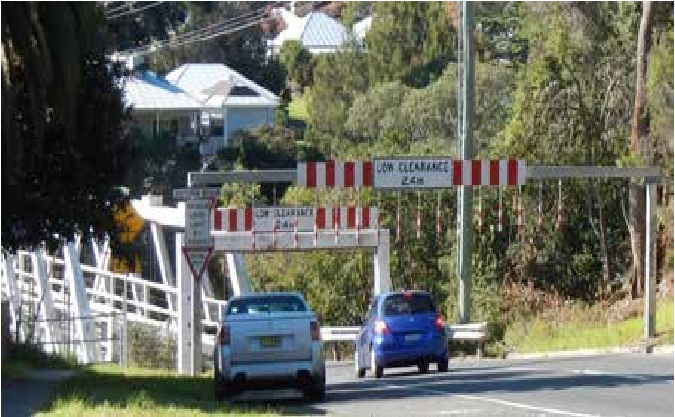
Figure 2-53: Height restriction portals
