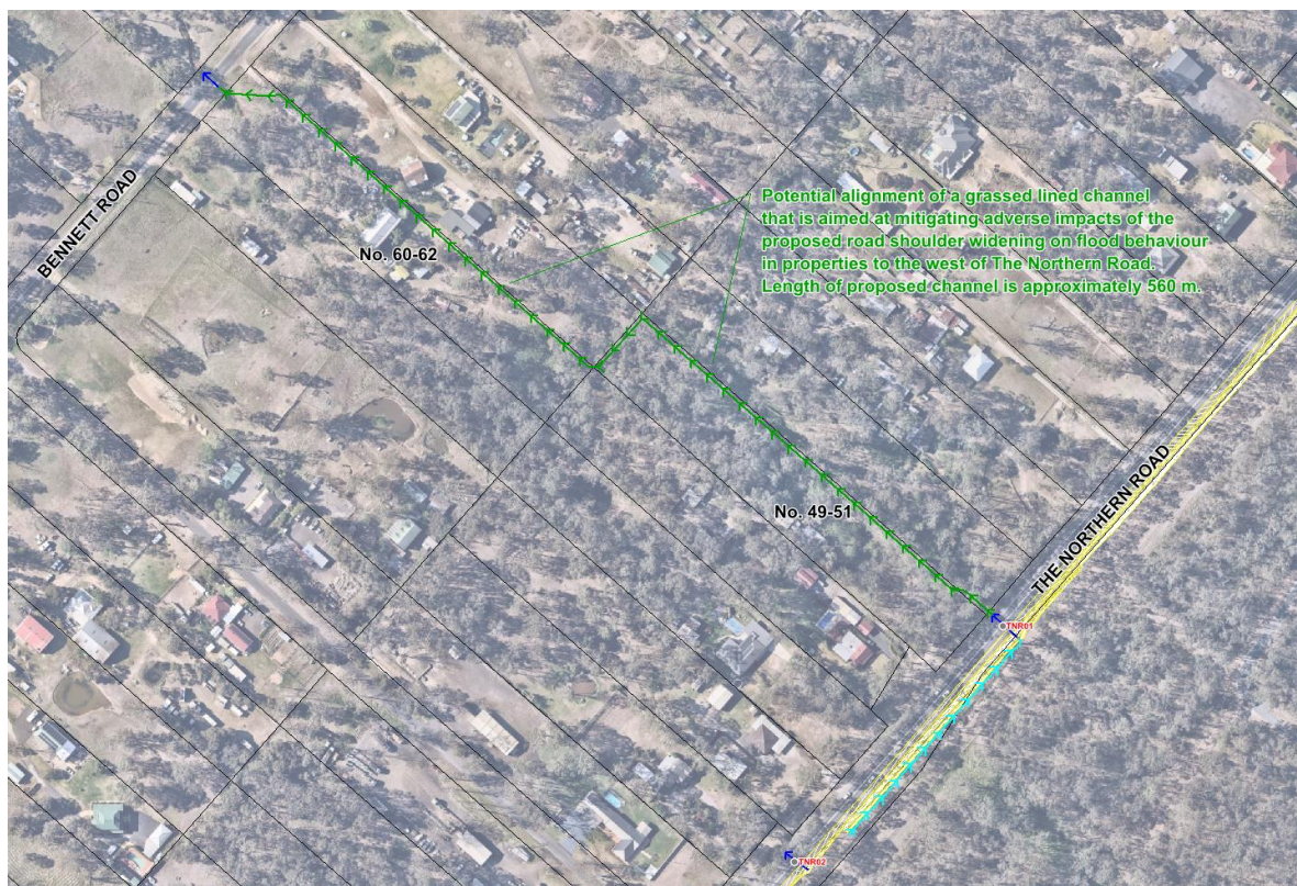
Plate 6.1 – Alignment of potential flood mitigation channel downstream of transverse drainage structure TNR01
