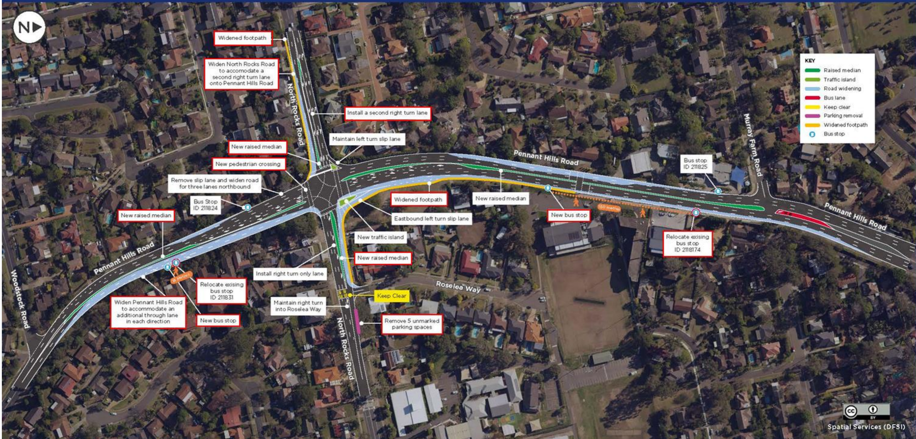
Figure 1-3: The proposed modification (subject to detailed design). Proposed modifications are outlined in red.
