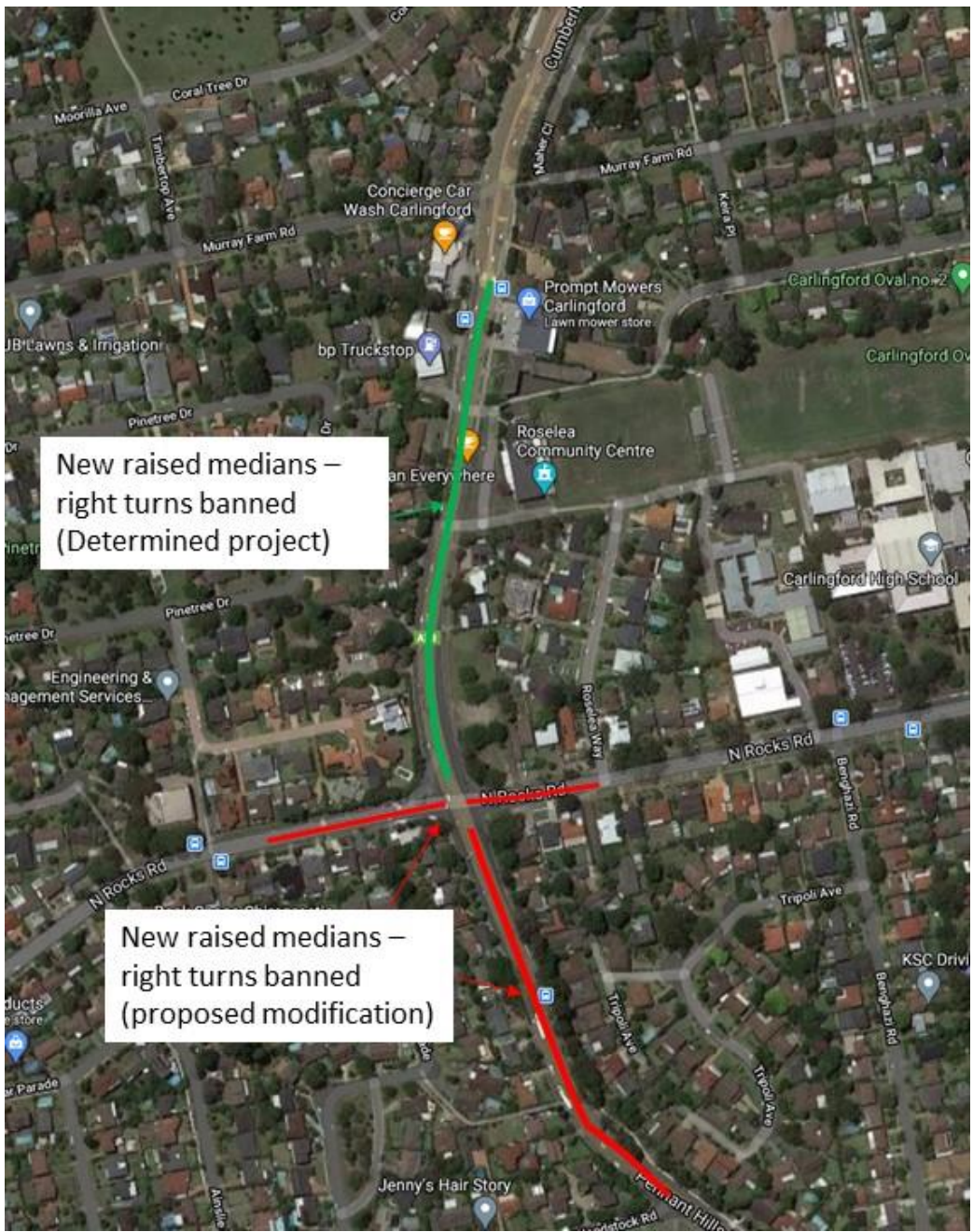
Figure 6-8 Location of new raised medians which would prevent right turns into property accesses
