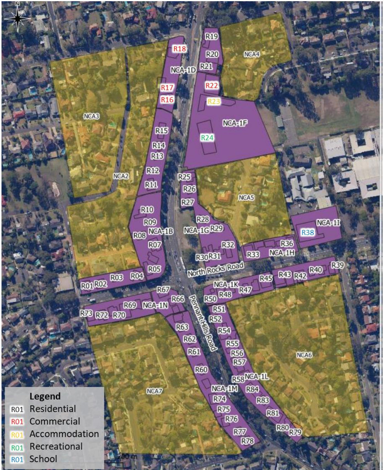
Figure 6-2 Site plan identifying Noise Catchment Areas and sensitive receivers considered Measured noise levels
