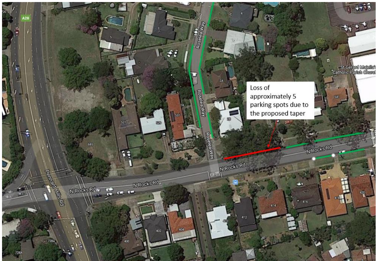
Figure 6-13 Location of parking spaces proposed to be removed are shown in red. Available unrestricted offset parking is shown in green.
