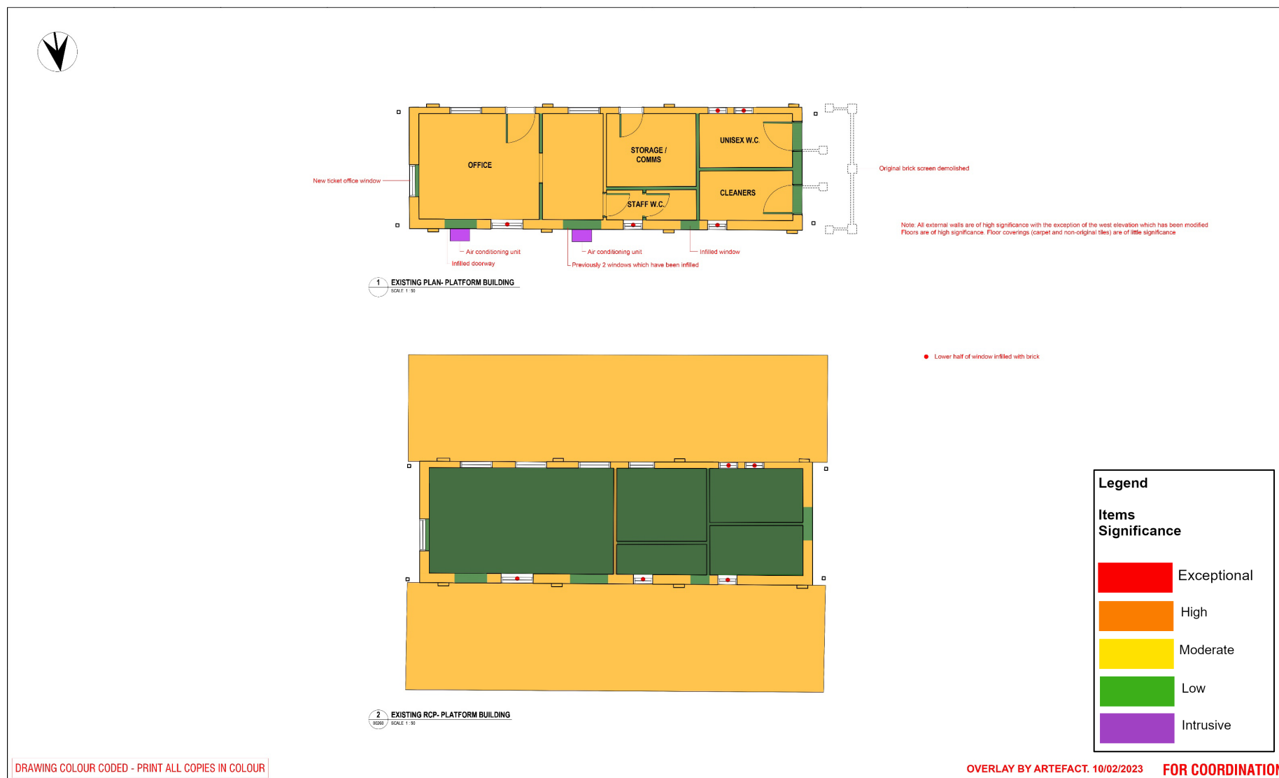
Figure 70. Gradings of significance – existing floor plan of the platform building and reflected ceiling plan, not to scale (Source: HDR [Design Inc with Artefact overlay]).
