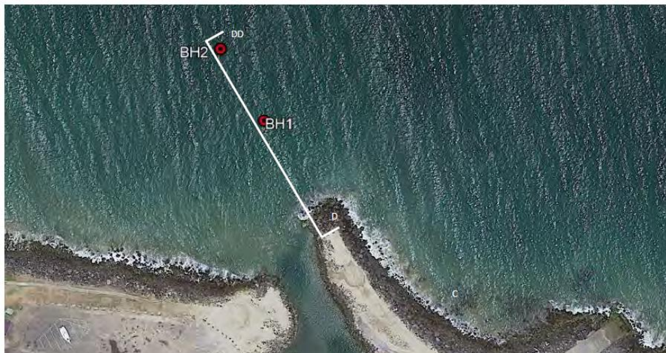
Plate 3-1: Coffs Harbour Regional Boat Ramp Geotechnical Investigation boreholes (RGS, 2020)
