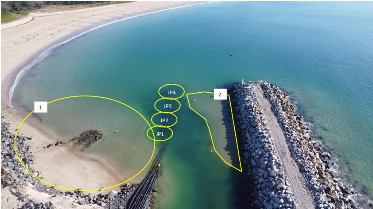
Figure 1 Location of existing sand transfer pumps within the boat ramp entrance channel (JP1 - JP4)
