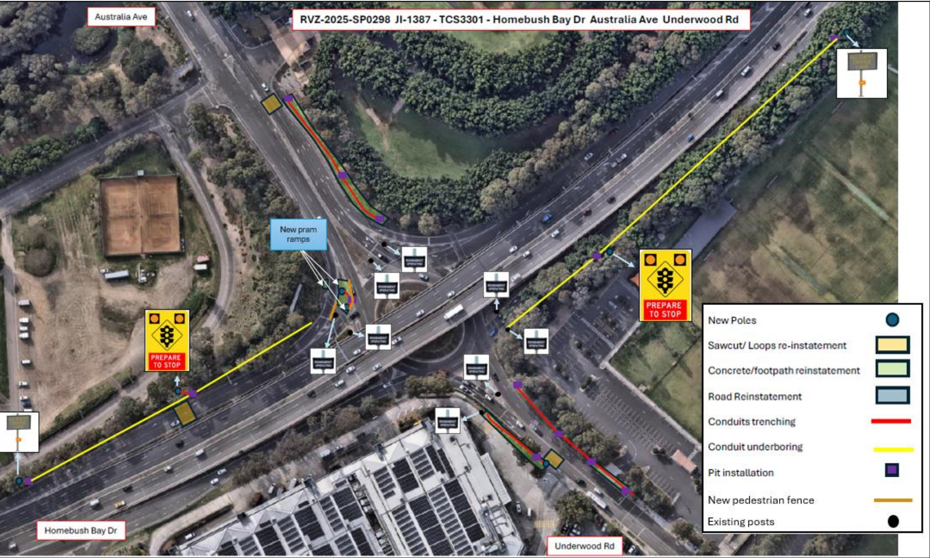
Figure 2.3 - Proposed upgrading works at the intersection of Homebush Bay Drive, Australia Avenue and Underwood Road
