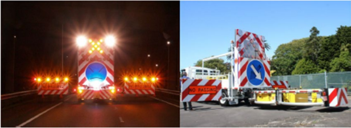
Figure 4.3 TMA host vehicle with outriggers deployed (source: Waka Kotahi NZ Transport Agency, 2021)
