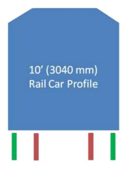
On the right is an example of a container profile on a 3040 mm width Freight Rail tray / car.
