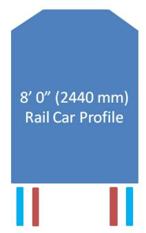
It should be very obvious that Isambard Brunel's "Broad" railway gauge would be far more stable than the "Standard" rail gauge for these 8' 0" (2440 mm) width Rail Cars.
