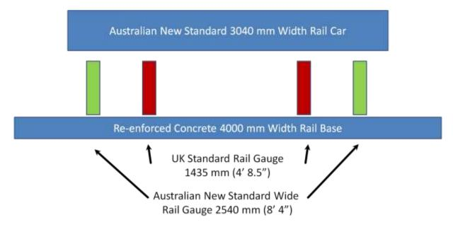
The above picture is typical of the lateral cross section of a 3040 mm (10') width Rail Car base with the option of the "UK Standard Rail Gauge" - in rusty red, and the "New Australian Standard Wide Rail Gauge" shown in lime green, with a 4000 mm (13' 7.5") width re-enforced concrete sleepers / rail base. It is clearly obvious that the "Australian Standard Wide Rail Gauge" will provide a far more stable load support than the inappropriate ancient CE 1820 - 1846 UK Standard Rail Gauge.
