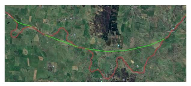
The above map is in central NSW where there are "rolling hills" and the course of the existing (single line) railroad is show in "rusty red" as it circumnavigates hill and runs around valleys - where an almost straight through "saddle cut" (as shown as a lime green line) indicates where the rail could (easily and inexpensively) be run.
