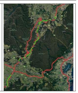
By using Heavy Earth Moving machinery, most of these tight arc rail lines can be substantially straightened to have radii exceeding 4 km. At the southern end of the map the line south of Moss Vale – near Exeter can also be substantially straightened.
