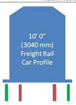
With the Standard Rail Car Width of 3040 mm (10' 0"), Containers (that have a standard width of 8' 0" (2440 mm) and motor vehicles can comfortably sit in a 10' (3040 mm) width rail car and be quickly / properly secured - and be "wind / stone shielded"!
