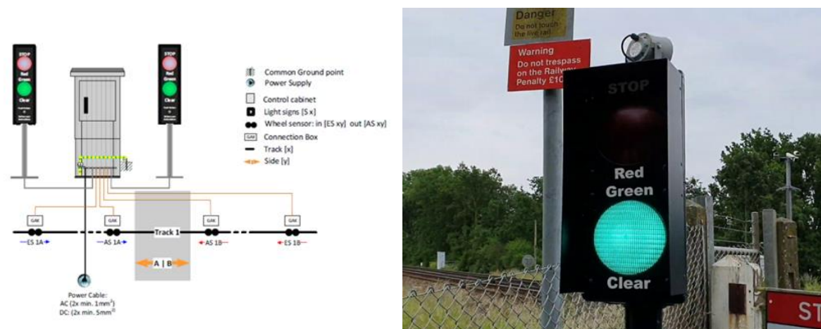
Figure 12: Typical Vamos level crossing signalling components for a private level crossing.
