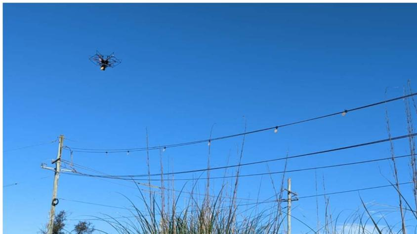
*Drone installing bird diverters on powerlines*
