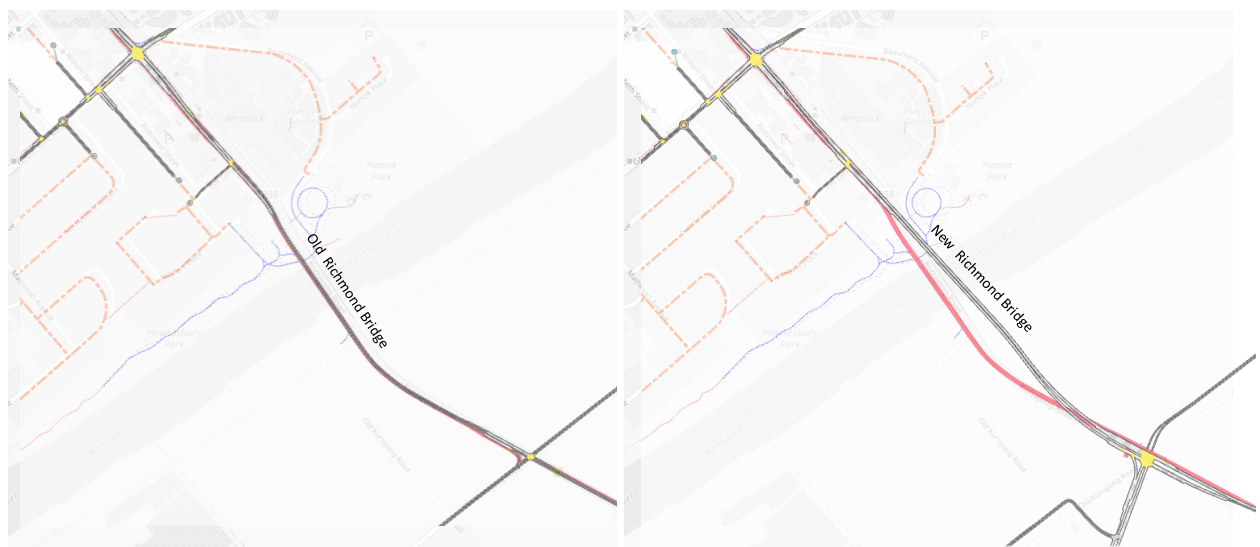
Figure 2-6 Existing Richmond Bridge alignment (left) and the new 4-lane Bridge over Hawkesbury River (right) (Location 2)
