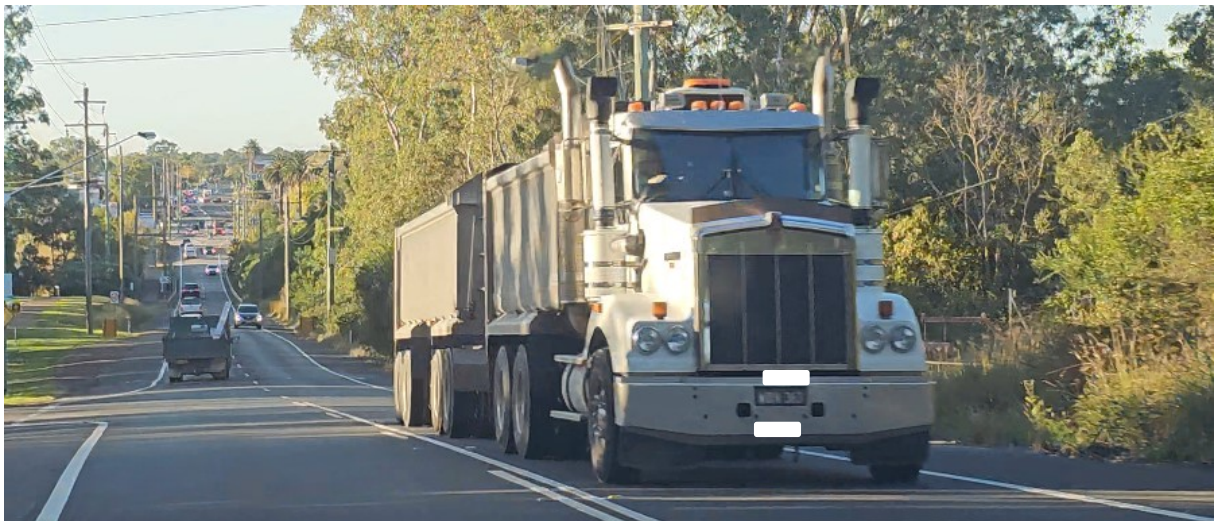
Figure 9: Rigid truck and trailer combination (3-axle truck and 4-axle dog trailer)
