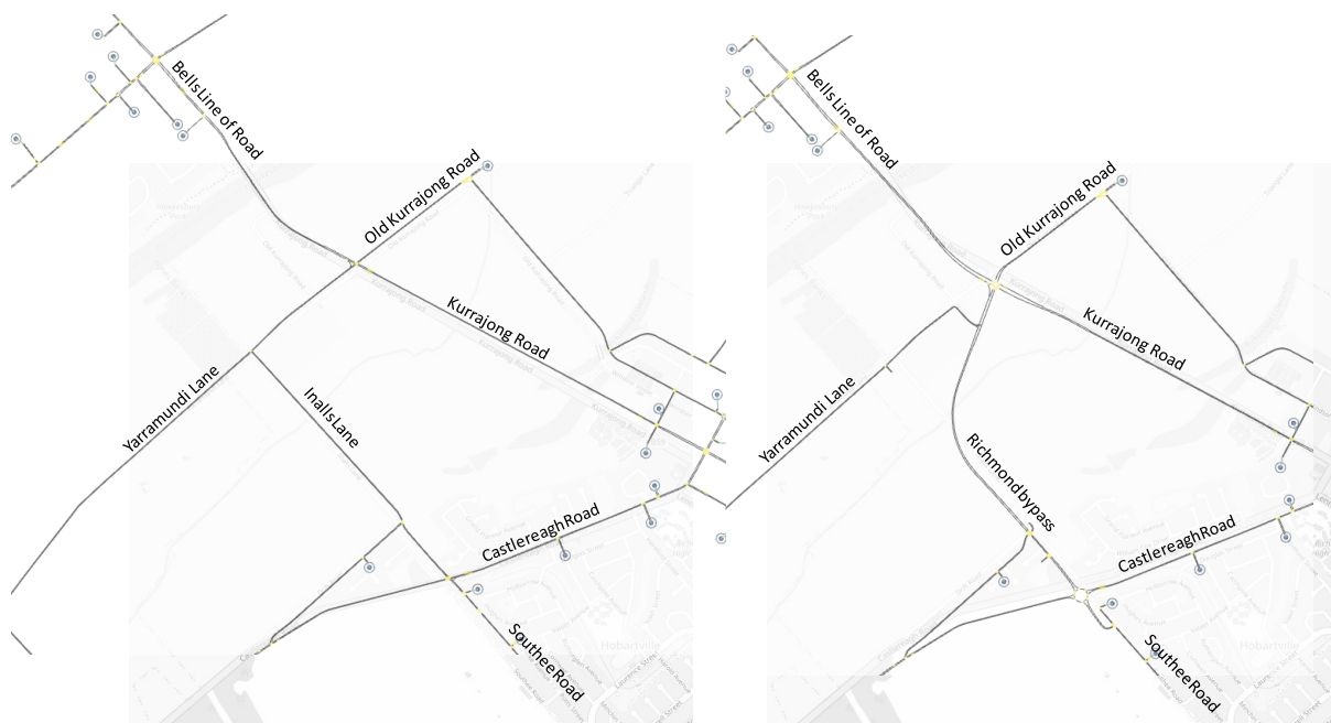
Figure 2-8 Existing network (left) and proposed Richmond bypass (right) (Location 4)
