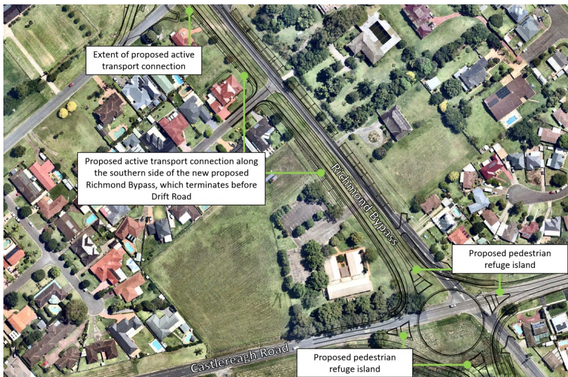
Figure 4-26 Proposed active transport connection at the new proposed Richmond bypass and Castlereagh Road roundabout intersection
