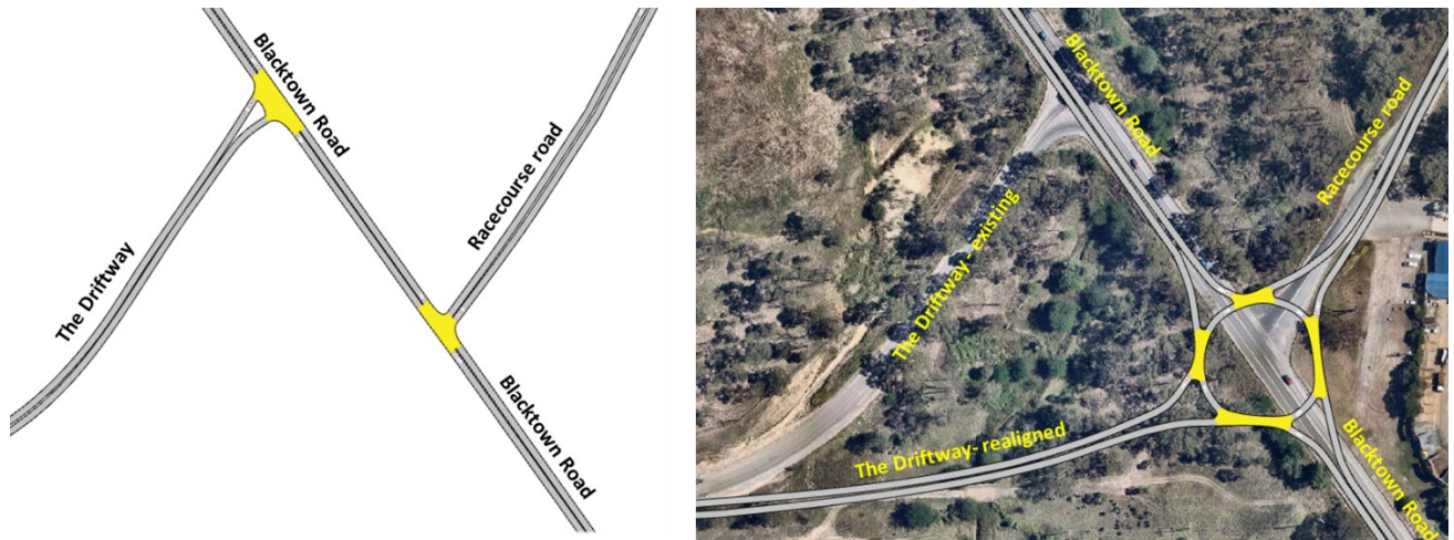
Figure 2-4 Blacktown Road, The Driftway and Racecourse Road intersection (Location 4) – existing layout (left) and proposed upgrade (right)
