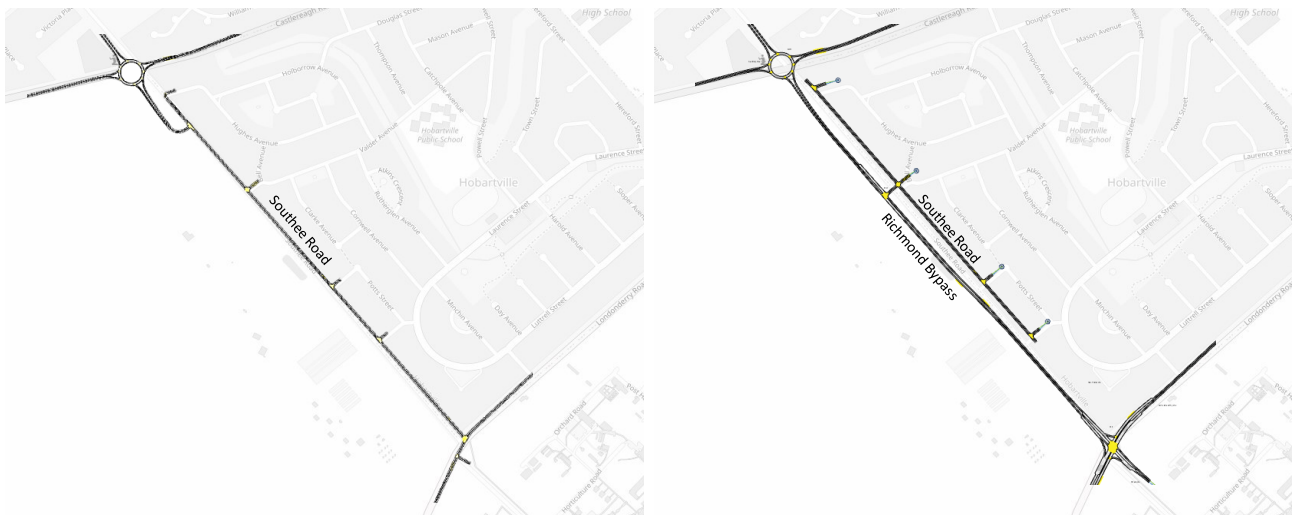
Figure 2-14 Richmond bypass along Southee Road (Location 9): Stage 2A Southee Road alignment (left) and proposed Richmond bypass (right)
