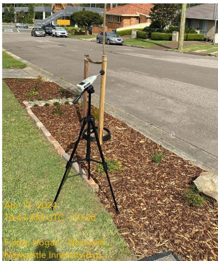
Figure 2-3 Attended noise monitoring
