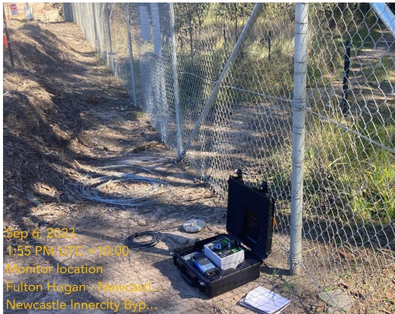
Figure 2-2 Attended vibration monitoring
