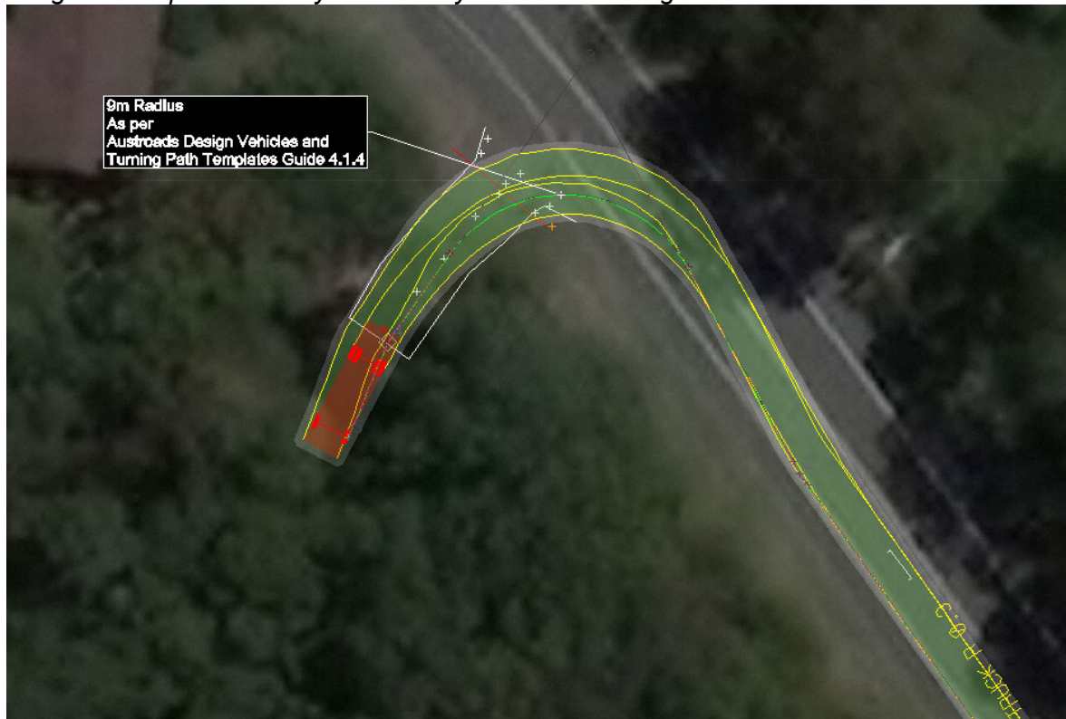
Image 2: Swept Path Analysis of heavy vehicles entering Marshall Street.
