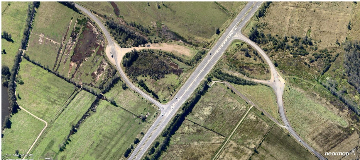
Figure 1-1: Pacific Highway (A1) intersection with Harrington and Coopernook Road - current at-grade 'Staggered-T' intersection arrangement (Nearmap, 2012)
