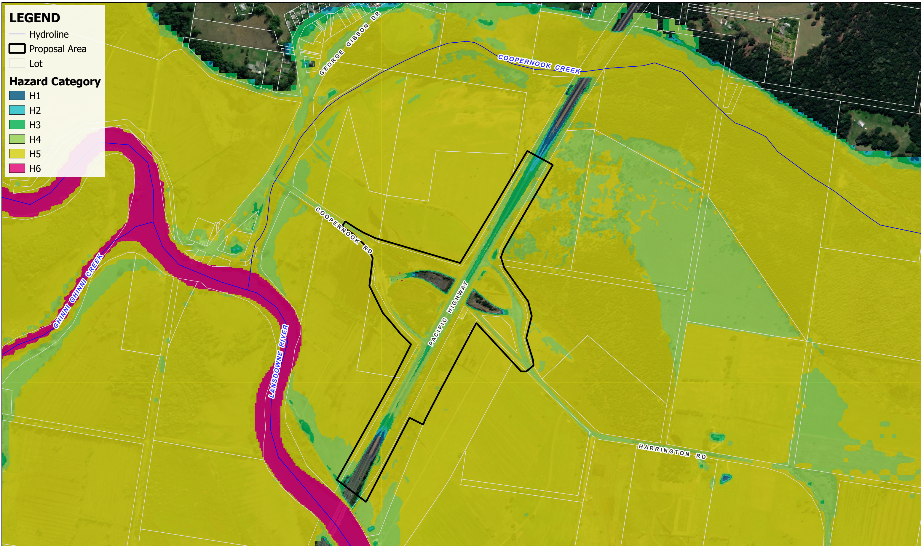
Title: Peak Flood Hazard - Existing Conditions - 1% (1 in 100) AEP Event with Climate Change
