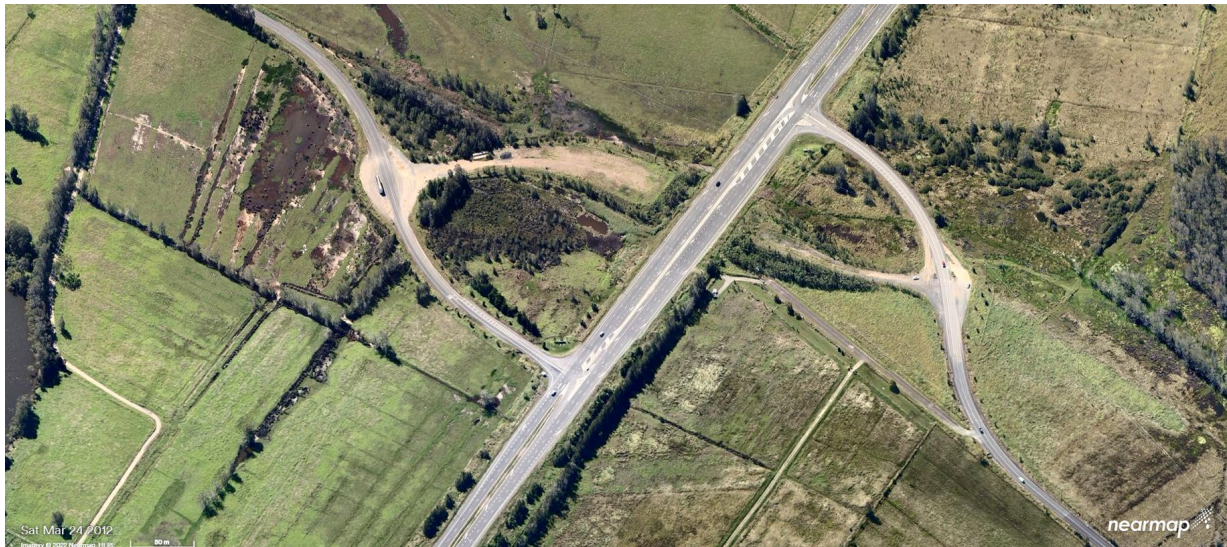
Figure 1: Pacific Highway (A1) intersection with Harrington and Coopernook Road - Current at-grade 'Staggered-T' intersection arrangement (Nearmap, 2012)
