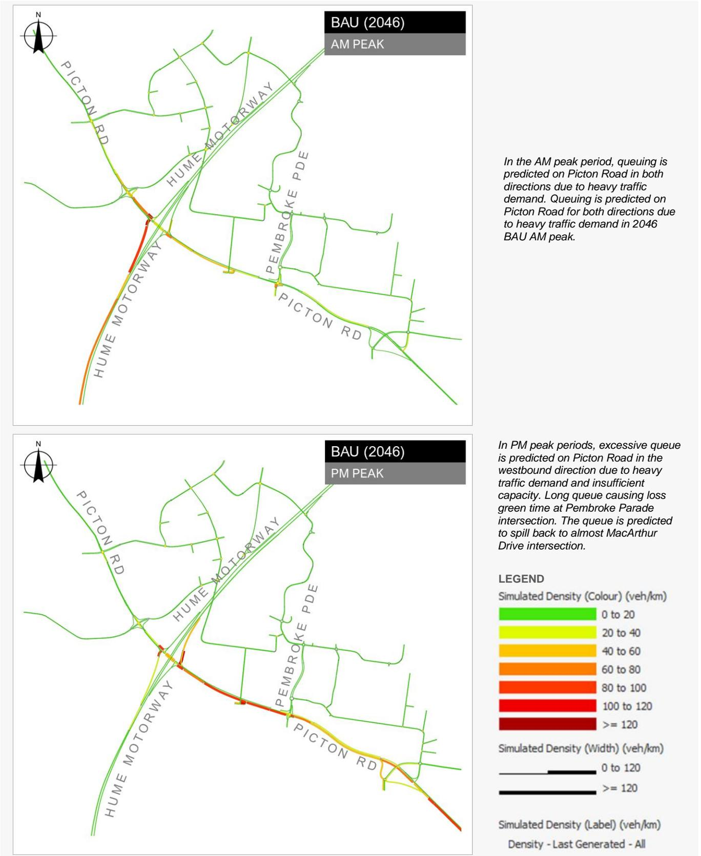
Simulated density in PCU/km/lane can be taken to be about 1.3 times the value shown on the plots above
