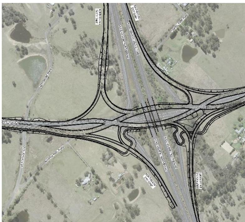
Figure 5.2 Proposed concept design: Picton Road and the M31 Hume Motorway interchange
