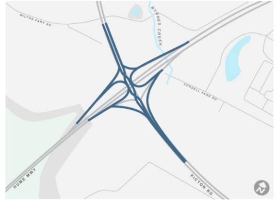
Diverging diamond interchange
