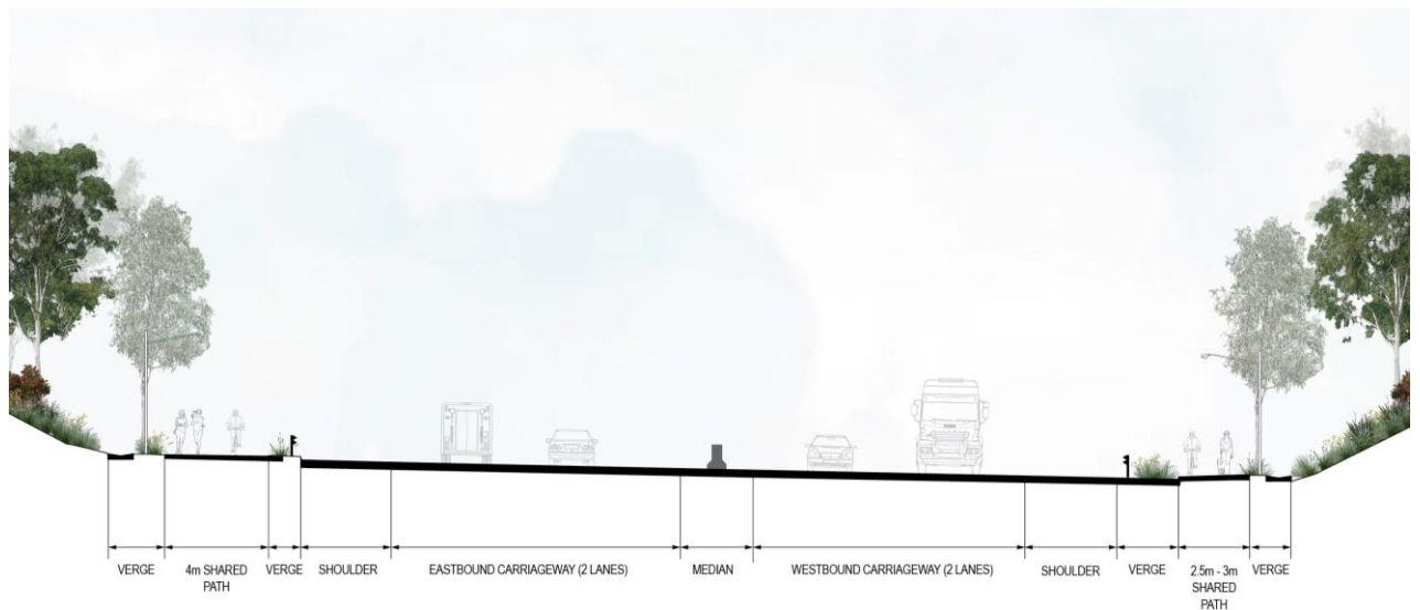
Figure 3-6: Typical cross section of Picton Road west of Wilton Park Road (two lanes in each direction) facing west
