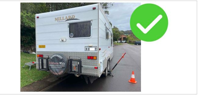
Tip-you must select an inspection area that is on a sealed hard level surface such as concrete or asphalt.
