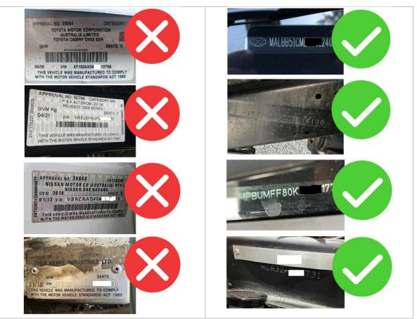
Tip – The photo must be of the stamped VIN or chassis number. A photo of the compliance plate or label is not sufficient.
