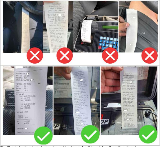
Tip – The photo of the brake test prints must be clear and legible and show the entire print out.
