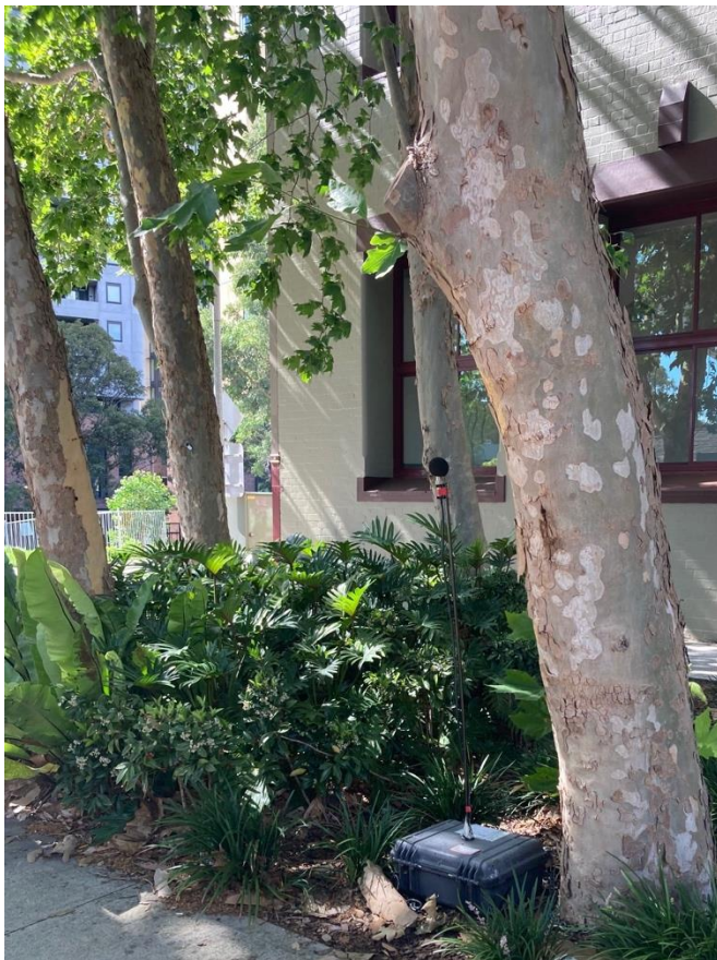
Photo 18 – Noise logger installed for operational noise monitoring.
