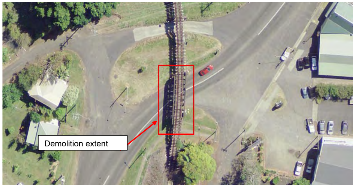
Figure E-6 Union Street Bridge – Demolition extent, spans 2 to 5 (Source: FBE)
