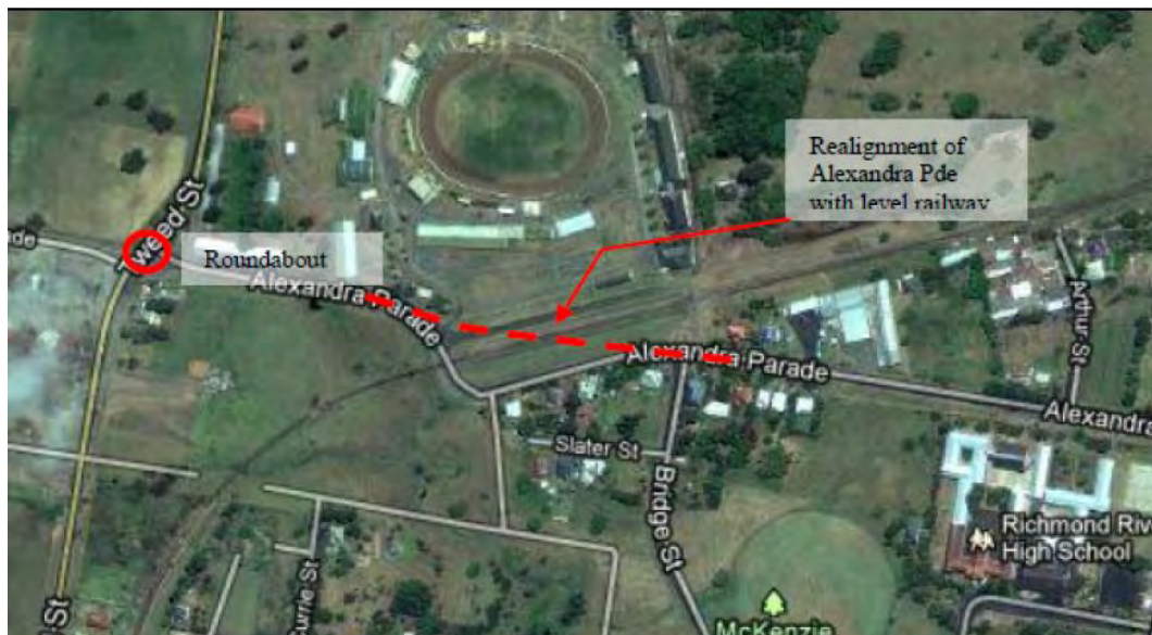
Figure 5: Potential realignment of Alexandra Parade to preserve railway bridge.
