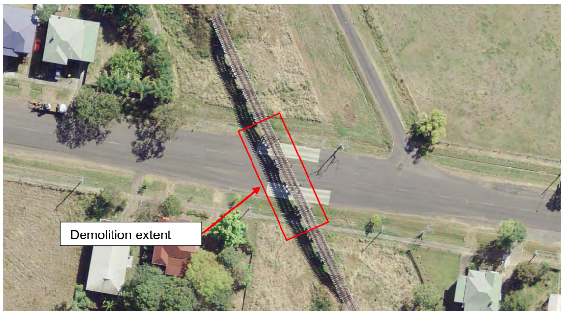
Figure E-5 Terania Street – Demolition extent, spans 4 to 8 (Source: FBE)
