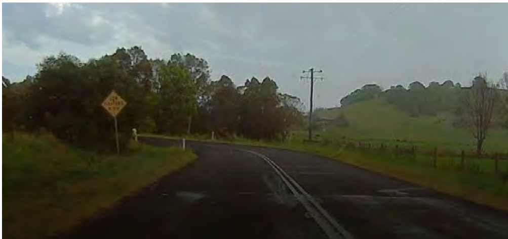
Photo 17: Inadequate definition of curve alignment – southbound approach to Winterton Parade viaduct
