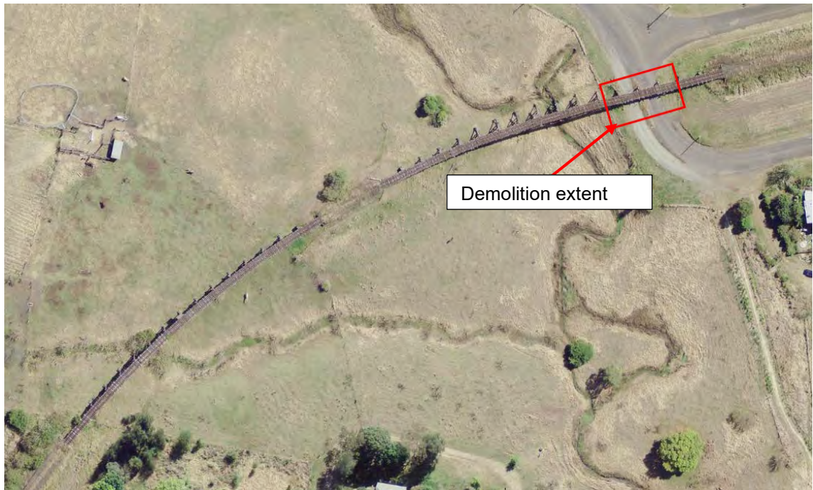
Figure E-4 Alexandra Parade – Demolition extent, spans 22 to 25 (Source: FBE)
