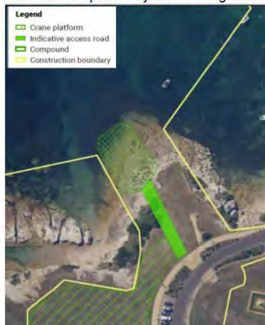
Figure 2-8 Temporary Crane Platform (La Perouse)
