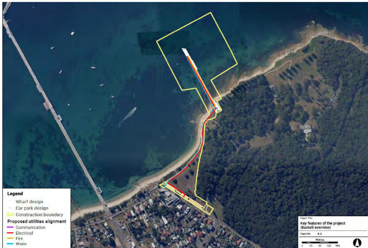
Figure 2-5 Construction Boundary and the Key Features - Kurnell
