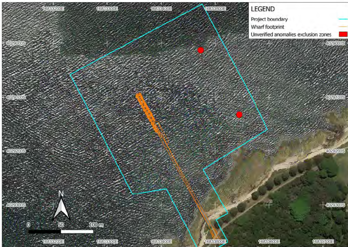
Figure B-8 Exclusion Zones (in red) of two unverified anomalies at Kurnell
