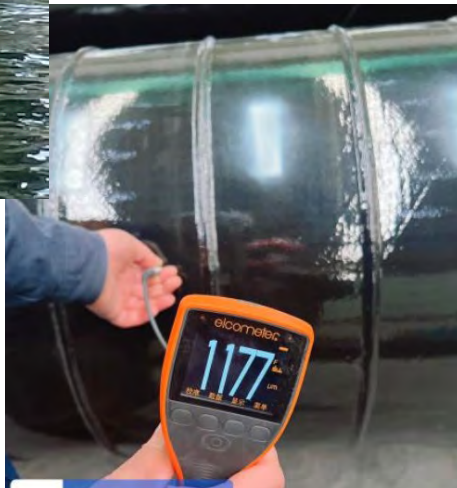
▲ Pile paint protection thickness testing
