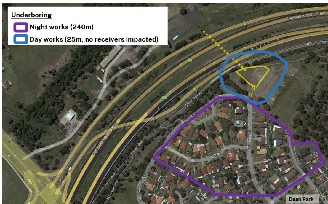
Figure 6-3: Construction noise impact map for Underboring works (receiver side). (Note, the night impact area reduces from 240m to 140m where there is no line of sight).
