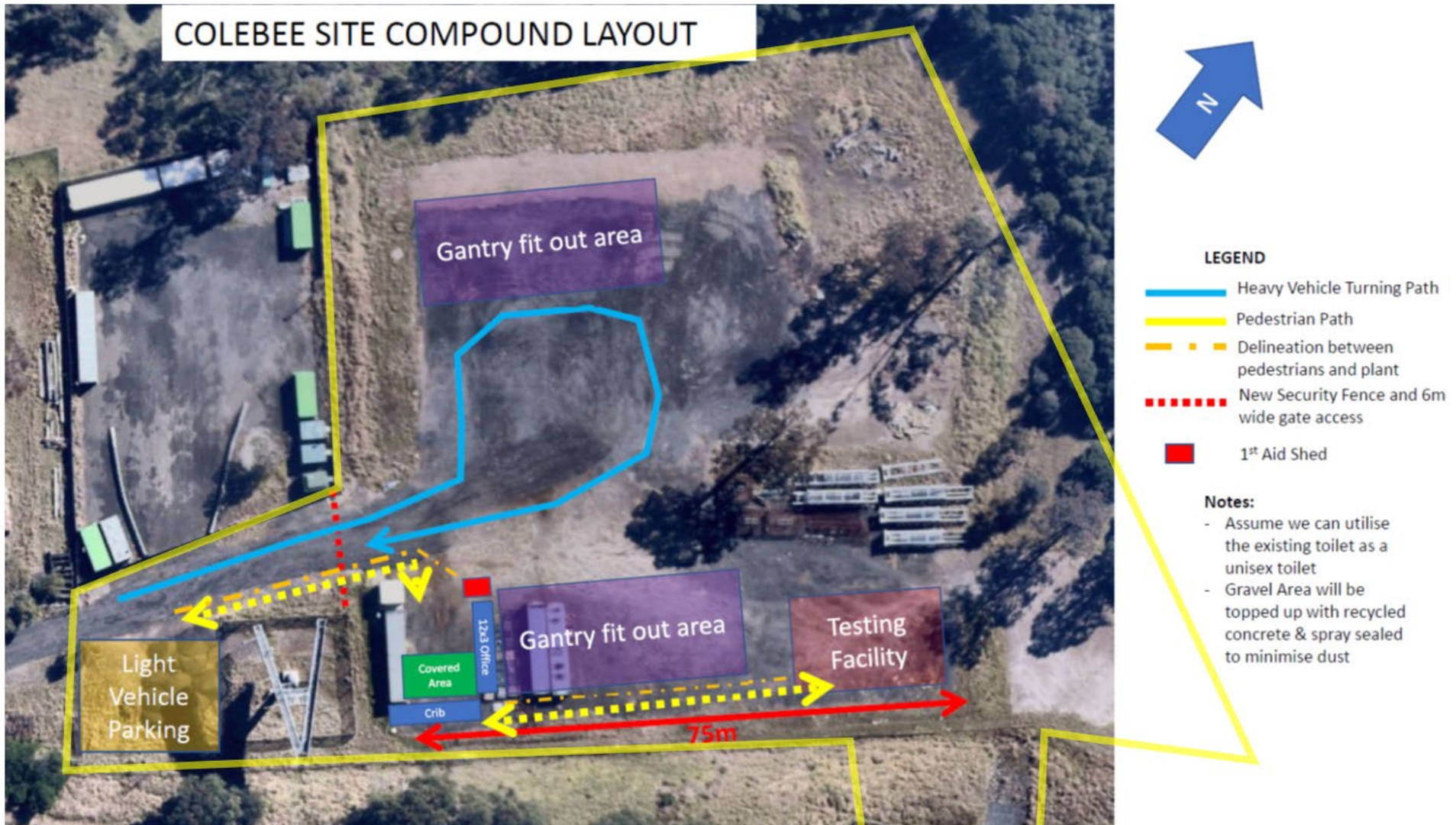
Figure 2: Potential construction compound layout plan
