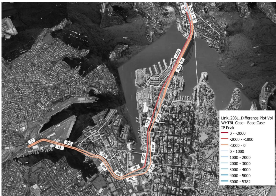
Figure 5.8: Difference plots of IP traffic volume between with or without WHTBL project, 2031
