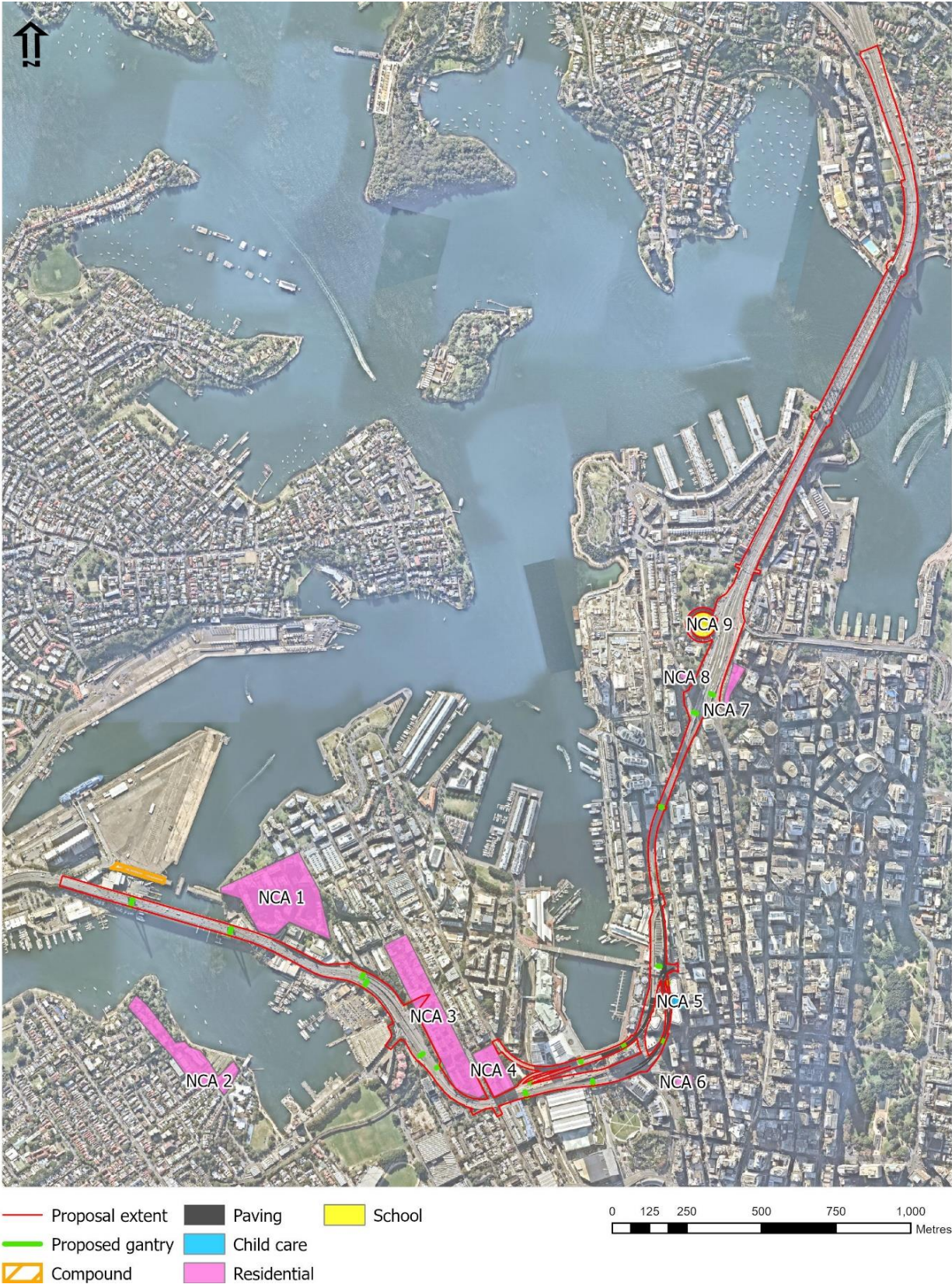
Figure 6-14: Location of noise sensitive receivers (worst affected) (Note: this figure depicts an outdated proposal area. Refer to Figure 1-2 for an accurate proposal depiction)
