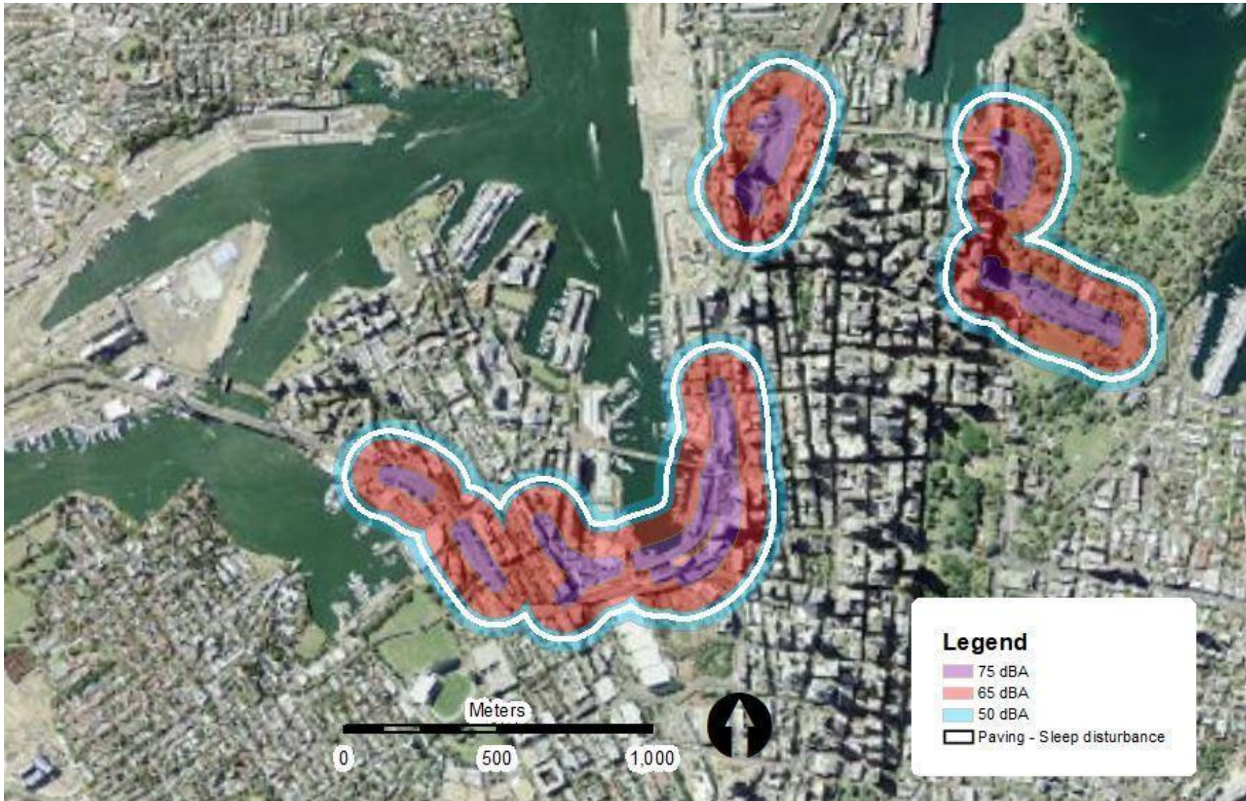
Figure 7: Paving / asphalting works assessment – Night
