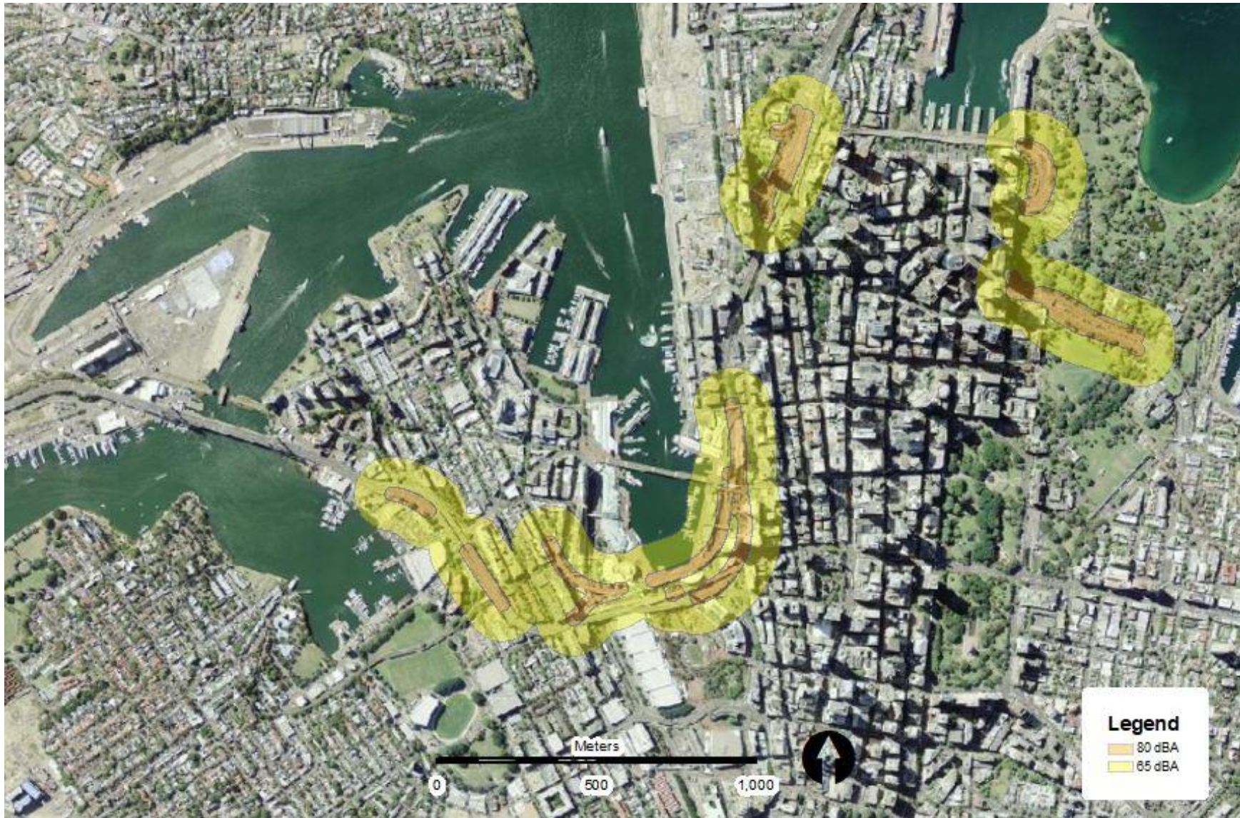
Figure 5: Paving / asphalting works assessment – Day (OOHW)
