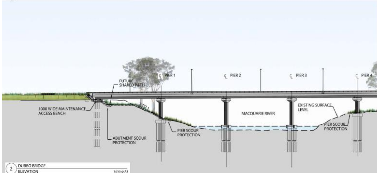
Figure 3-3 Proposed modified pier arrangements across the New Dubbo bridge
